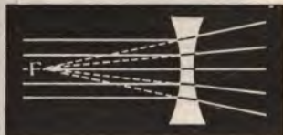
FIG. 152.—The Action of a Concave Lens on Parallel Rays.
